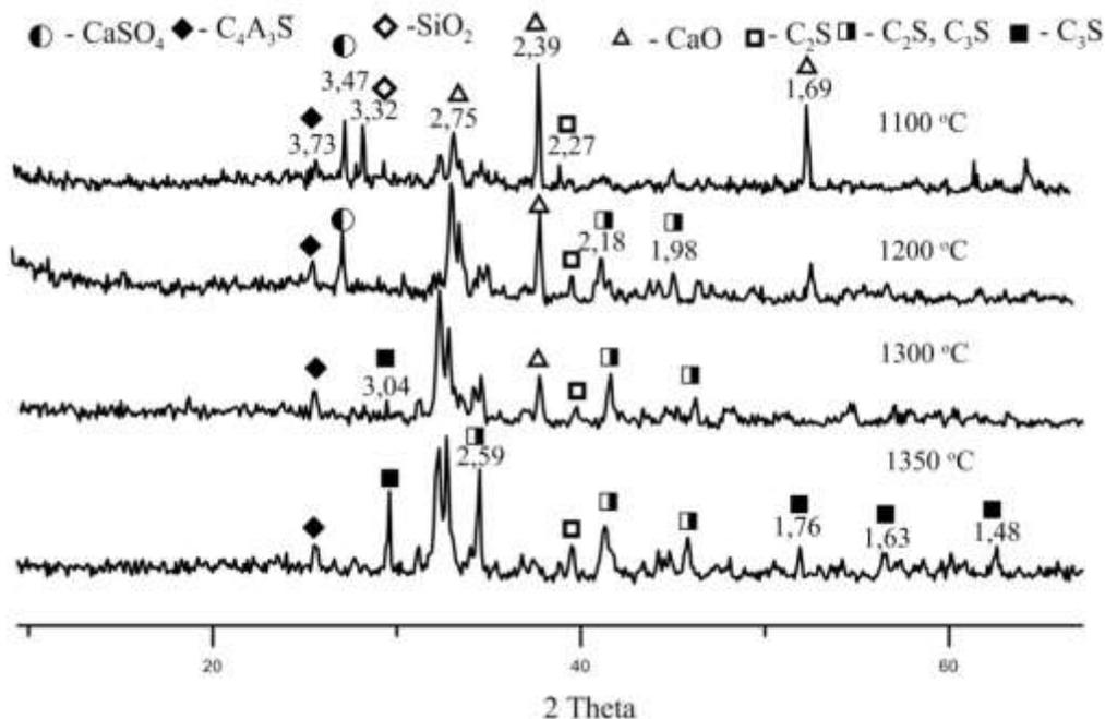
**Figure 6:** Results of qualitative x-ray analysis of clinker, prepared according to the calculation, given above and calcined at temperatures of 1100,1200,1300 and 1350 ° C.
