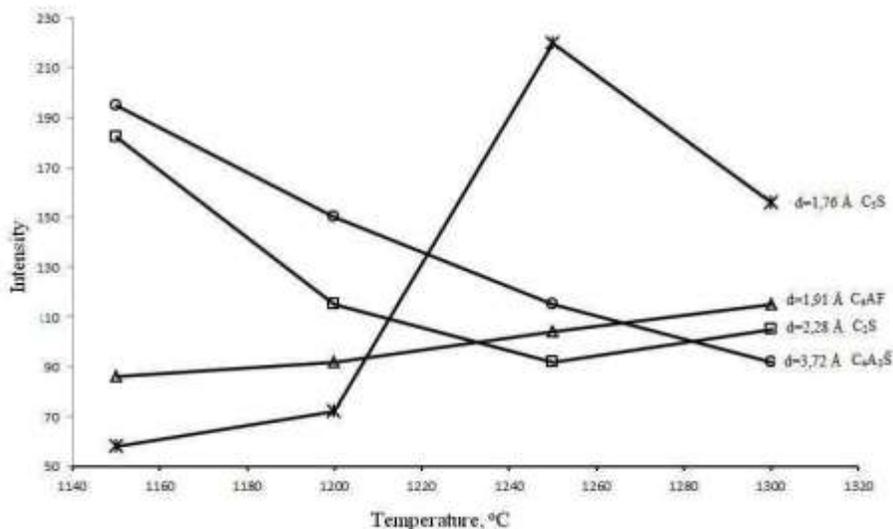
**Figure 3:** Intensity change diffractional maxima of the basic phases of clinker № 1 depending on roasting temperature
