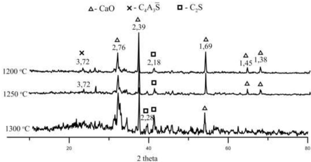
**Figure 1:** Results qualitative x-ray analysis of clinker with the additive 5 % of gypsum
