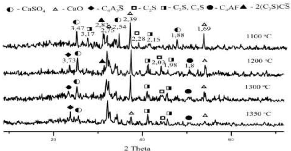
**Figure 5:** Results of qualitative x-ray analysis of clinker with metastable phases C<sub>4</sub>A<sub>3</sub>S̄ and 2(C<sub>2</sub>S)C̄S̄ calcinated at temperatures 1100,1200, 1300 и 1350 °C
