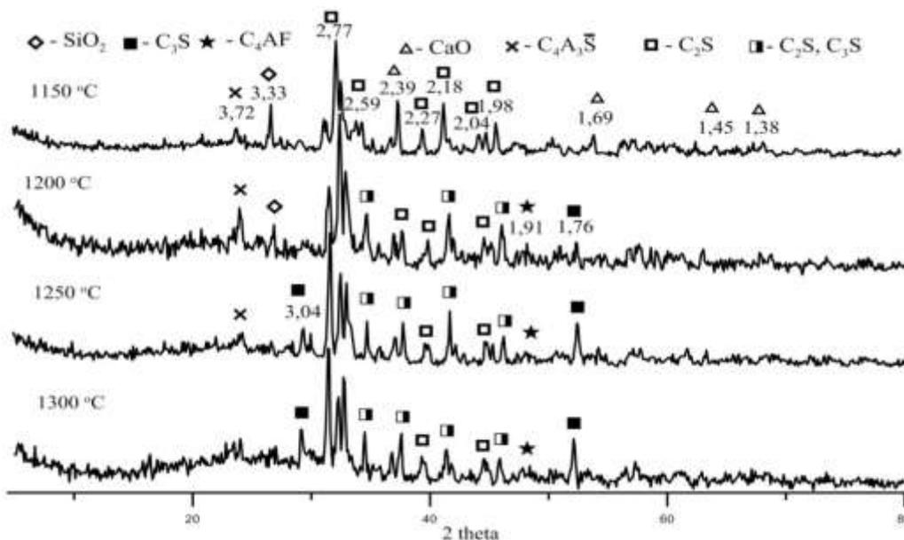
**Figure 2:** Results qualitative x-ray analysis of clinker № 1, calcinated at temperatures from 1150 to 1300 °C
