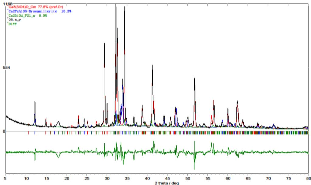
**Figure 4:** Results of quantitative x-ray the analysis for clinker № 1
