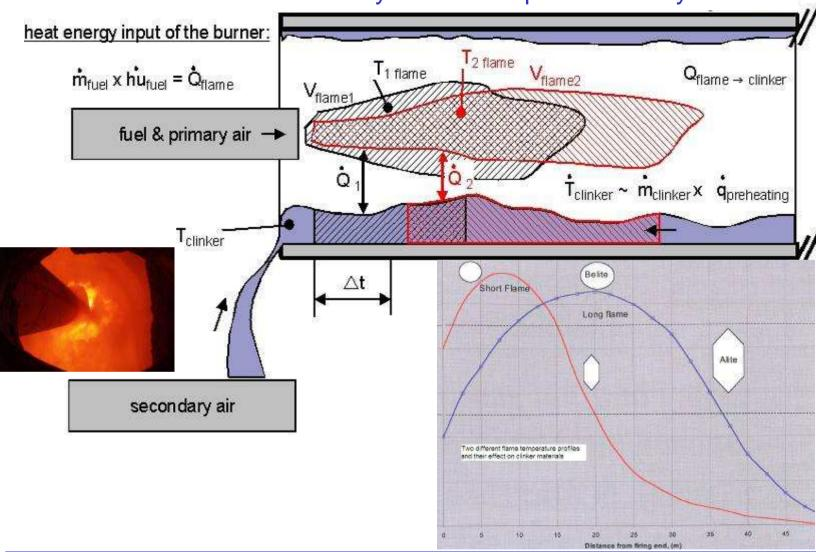
Flame geometry, the basis for enhanced process transparency
