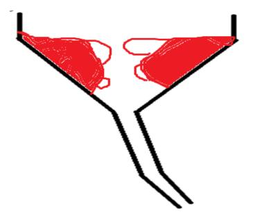
cone draft point just above 1.5 mtr height from discharge point when feed stopped on that time cone draft was negtive. after checking feed pipe and cone discharge there was no material in this area but material was in cyclone. causes of this ......?
