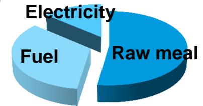
➤ Actual CO<sub>2</sub> emission depend mainly on clinker factor and process efficiency, ranging from 0.7 to 1.1 t CO<sub>2</sub> per t-cement globally;
