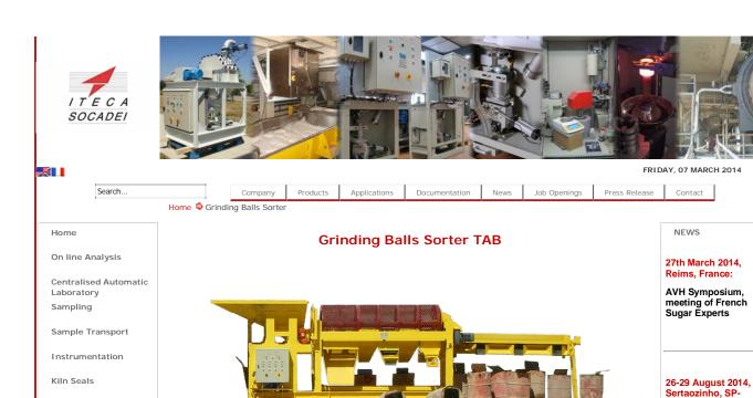
THE GRINDING BALL SORTER ALLOWS THE AUTOMATIC SEPARATION OF BALLS, CYLPEBS, DUST AND SCRAPS
