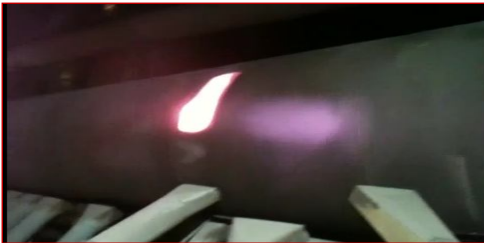
Figure-3: Red spot with 830°C temperature
